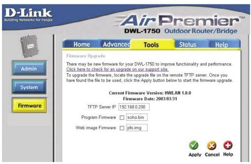
You can upgrade the firmware here. Make sure the firmware you want to use has been copied into the TFTP folder on the computer in your network which has the TFTP software installed. Remember the names of the firmware upgrade files. Please check the D-Link support site for firmware updates at http://support.dlink.com. You can download firmware upgrades to your hard drive from the D-Link support site.
